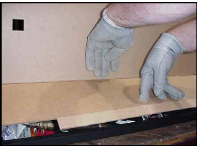
Figure 13.8 Opening Lower Access Panel
