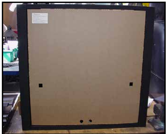
Figure 13.11 Splatter Guard with Lower Access Panel Closed
