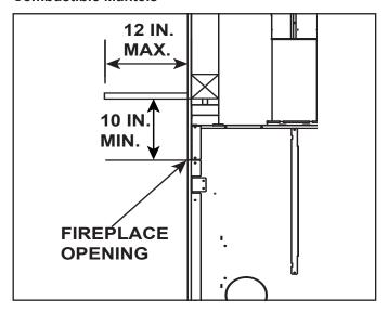
Figure 5.3 Clearances to mantels or other combustibles above appliance
