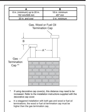
Figure 6.2 Staggered Termination Caps
