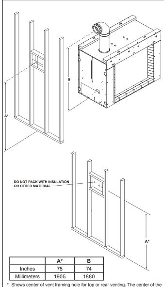
hole is one (1) in. (25.4 mm) above the center of the horizontal vent pipe.
