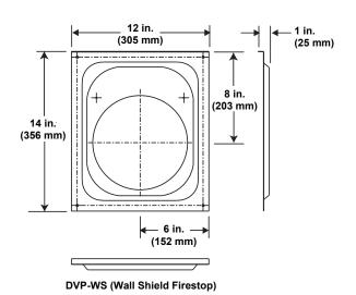
Figure 16.2 DVP vent components
