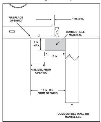
Figure 5.5 Clearances to Combustible Mantel Legs or Wall Projections.
