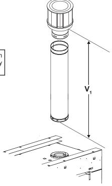
$V_1 = 50$  ft. Max. (15.2 m)  $V_1 = 3$  ft. Min. (914 mm)
