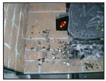
Figure 14.22 Ember Placement on Base Refractory
