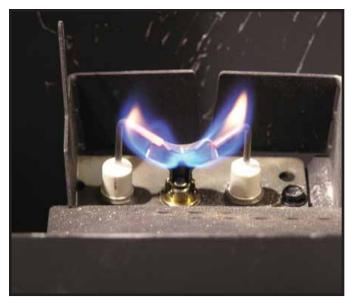
Figure 3.1 IPI Pilot Flame Patterns
