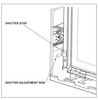
Figure 14.28 Shutter Adjustment Rod and Shutter Stop
