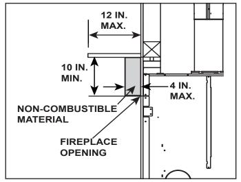
Figure 5.4 Clearances to Mantels or other Non-Combustibles Above Appliance
