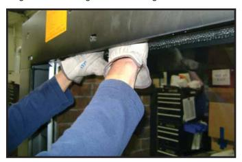
Figure 14.6 Top Glass Latch Access
