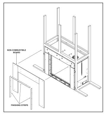
Figure 9.6 Attaching Non-Combustible Board
