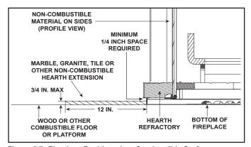
Figure 5.7 Fireplace Positioned on Combustible Surface
