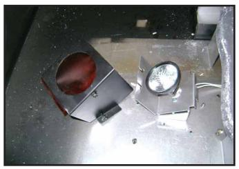
Figure 14.12 Light Housing Removed, Bulb Installed
