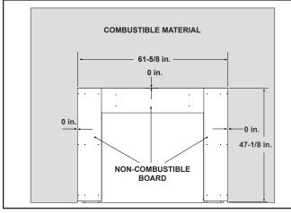
Figure 13.6 Noncombustible Facing Diagram
