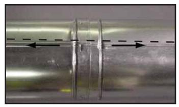
Figure 10.11 Align and Disassemble Vent Sections
