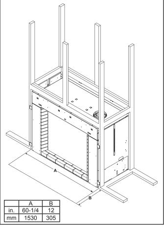
Figure 5.10 Non-Combustible Hearth Extension Minimum
