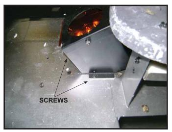
Figure 14.11 Light Housing Removal
