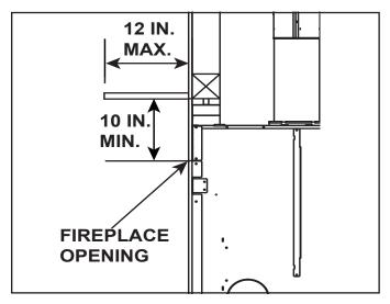
Figure 13.1 Clearances to Mantels or Other Combustibles
