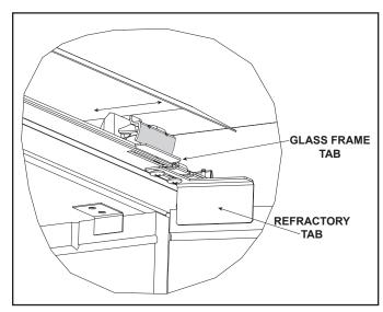
Figure 14.7. Top Glass Latch Detail
